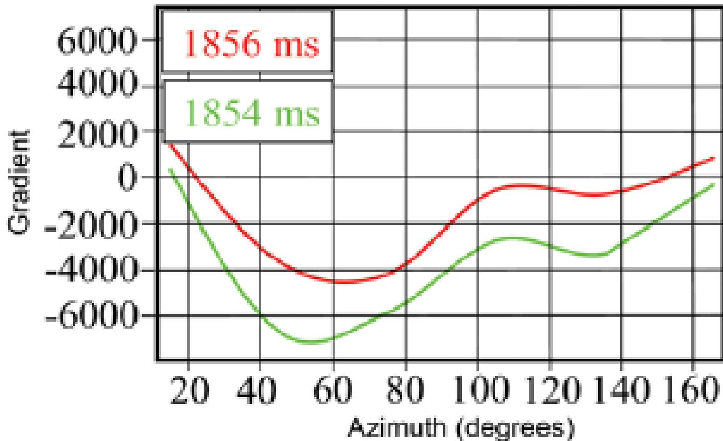
*Figure 4. Amplitude of the AVO gradient versus azimuth observed for a reflection from the top of the Falher Formation. The red curve was extracted at 1856 ms, and the green curve at 1854 ms. For an isotropic half-space overlying an HTI medium, the curves should exhibit a  $\cos^2(\phi)$  variation. The fact that they don't suggests a more complex fracture pattern.*
