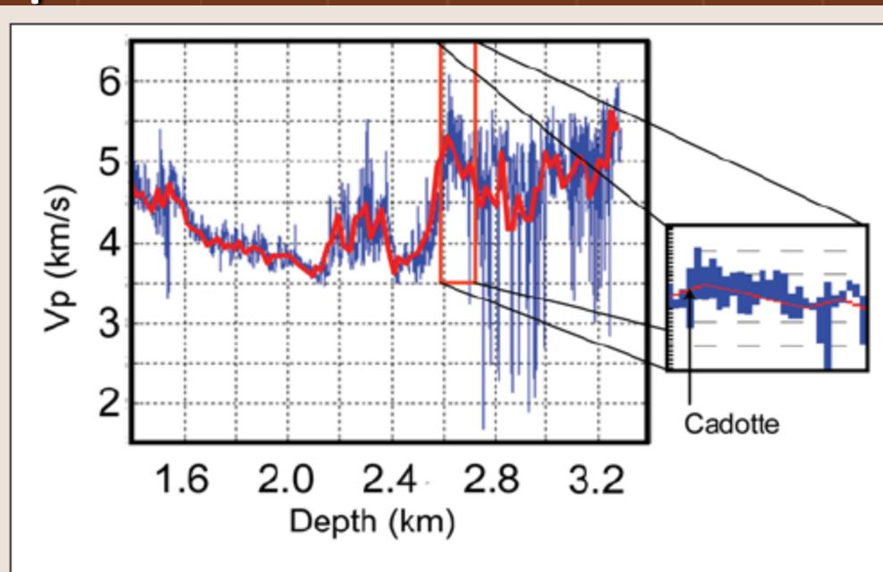
*Figure 5. Compressional-wave velocity log used for generating synthetic seismograms. The blue curve represents the recorded data, and the red curve the data used for generating synthetic seismograms. The actual location of the Cadotte Formation is shown on the inset.*
