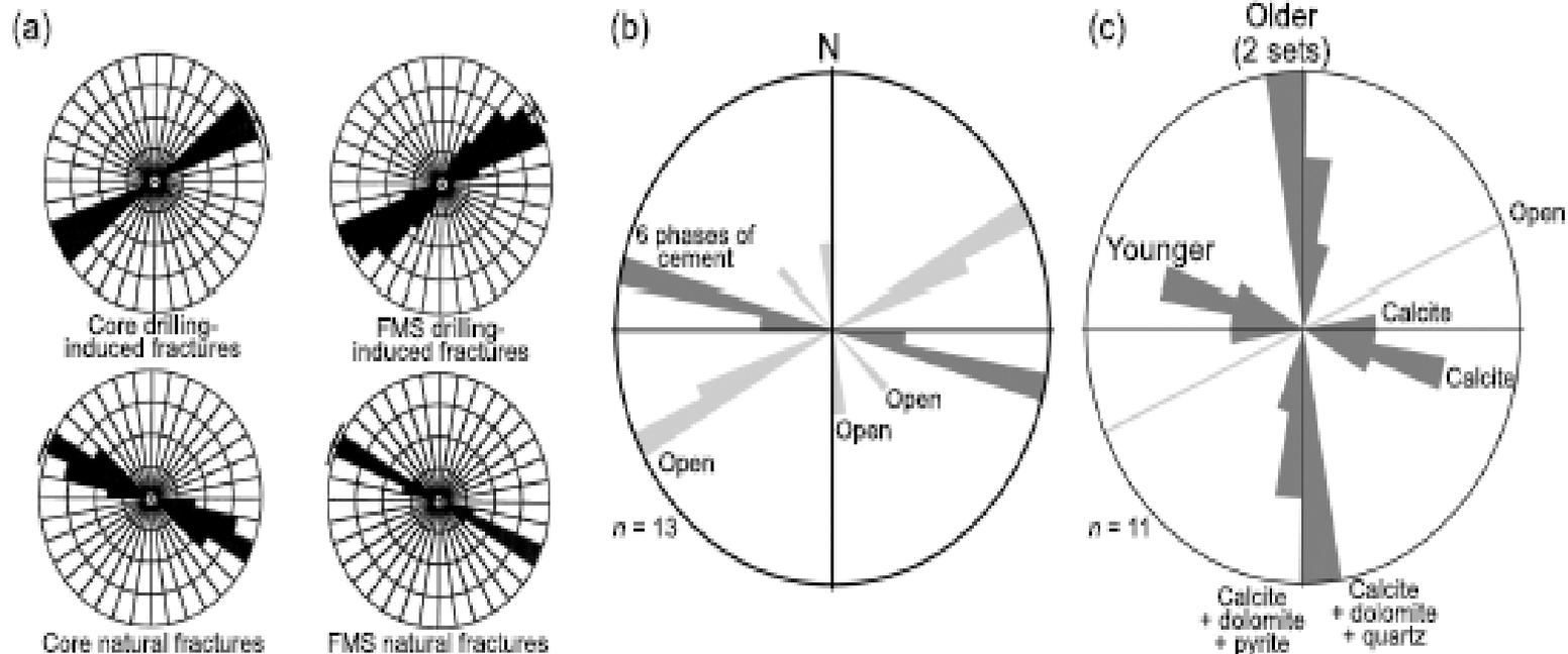
**Figure 5.** Rose diagrams showing fracture trends in the T. P. Sims core (a) from Hill (1992), used with permission from the Gas Technology Institute; (b) in the mudrock sample from this study; and (c) in the dolomitic sample from this study.
