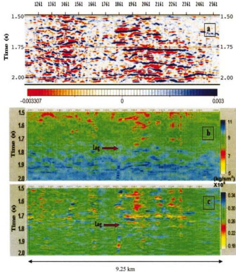
Figure 8. (a) Stacked seismic section for entire seismic line (CMP 1161 to CMP 2601) within a time window of 1.5–2.0 s. Blue color denotes positive amplitude, red denotes negative amplitude. Several anomalous zones are identified in (b) the acoustic impedance and (c) the Poisson's ratio.
