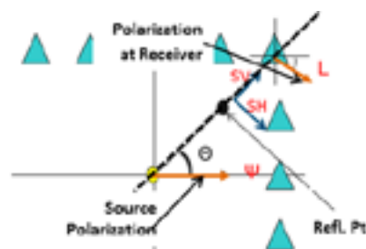
Figure 2. Acquisition configuration of source (center) a receiver (triangles) positions for a 3D direct horizontal shear-source survey.
