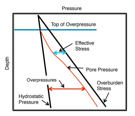
**Pore pressure** – pressure of fluid in the pore space of the rock
